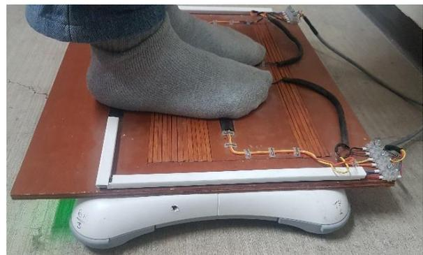
Figure 9. Simultaneous CoP measurement between proposed system and WBB.
