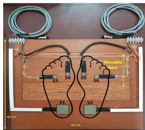
Figure 2. Platform with sensors and proposal press.
