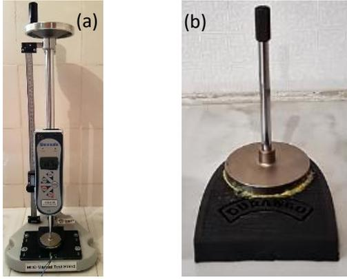
Figure 6. Elements for characterization of the sensor, (a) Dynamometer with bench and (b) Pressurizing rubber.
