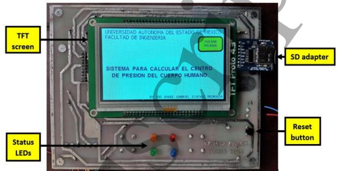
Figure 4. Electronic card of digitization stage.
